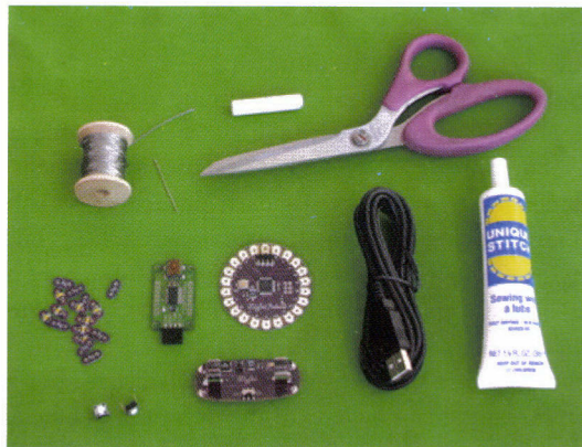
Figure 11.23 The LilyPad Arduino kit. It comprises sensors, actuator boards, and conductive thread. Online tutorials are available that enable anyone to build their own (see web.media.mit.edu/~leah/LilyPad/build/turn_signal_jacket.html )
